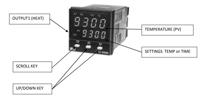
Left symbol "Scroll Key" is also used for configuring regulator parameters. **Observe great caution** when changing unit parameters. Incorrect programming (setup) can cause unit malfunction, incorrect temperature, or damage to the controller components.
