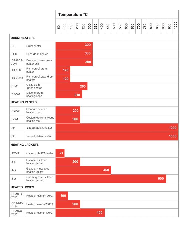
The datasheets here show our standard range of products. Use the table below to help select the right product. In the electronic version, click the item to go to the relevant datasheet. Our engineers have good capabilities to generate new electric heating solutions, so if what you need is not here, email isopad.info@thermocoax.com with your requirements.
